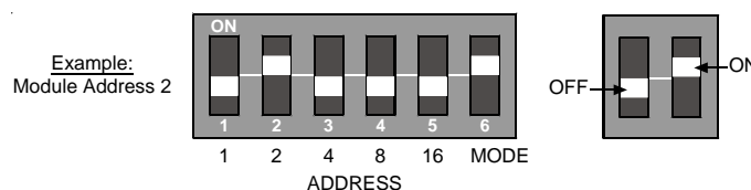
Figure 31: Command Center DIP Switch Orientation
